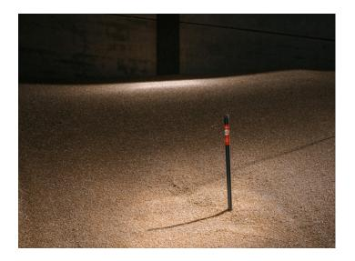
In practice, Javelot's Store&Save solution connects silos to collect key data such as temperatures, enabling the automation of ventilation using algorithms that trigger fans only when the temperature difference between outside air and grain is sufficient to produce actual cooling. Store&Save also issues alerts in case of overheating inside the silos, allowing silo managers and on-site operators to respond in time before insects start to develop.
